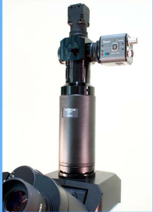
MV - 100% Vert / 100% Horz Multiport with 2x C-Mounted cameras
