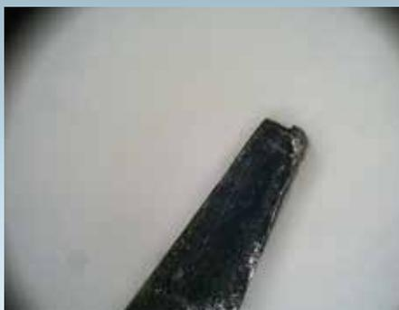
Deformation at the tip of the driver (SP-01 40x)
